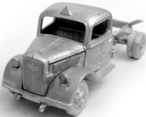
The bonnet and front grill are glued in place next. And you'll want to dry fit the cab roof to see how it looks - but it's a good idea to glue this piece last - especially if you want to paint the cab interior or fit the glass for the windscreen and side windows.
